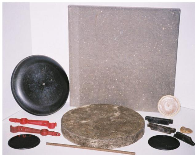
**Fig. 6.** Different plastic and resin products containing kenaf fibers.
