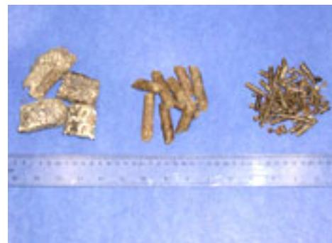
**Fig. 4.** Whole stalk kenaf compressed into small pellets (right), range pellets (center), and square cubes (left).
