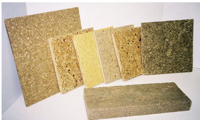
**Fig. 5.** Different types of building materials containing whole-stalk kenaf.
