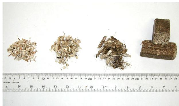
**Fig. 3.** Core fiber material; small (left), medium (second from left), large (third from the left), and compresses into a square cube.
