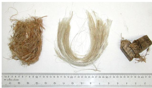
**Fig. 2.** Kenaf bark fiber strands; fiber strands after harvesting with a forage chopper (left), retted combed fiber strands (center), and fiber strands compressed into a square cube.
